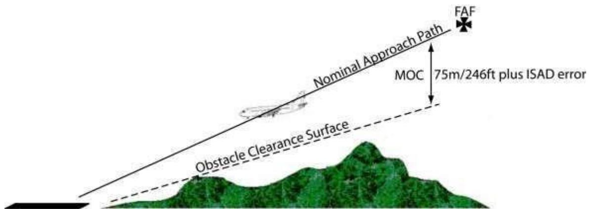
Figure 6.4: RNP APCH (LNAV/VNAV) Final Segment Obstacle Clearance
