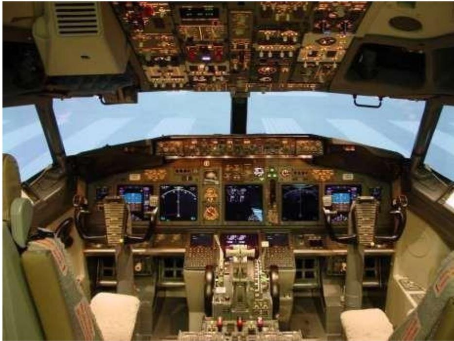
Figure 2.5: FMS Equipped Aircraft with Large Screen Multifunction Displays
