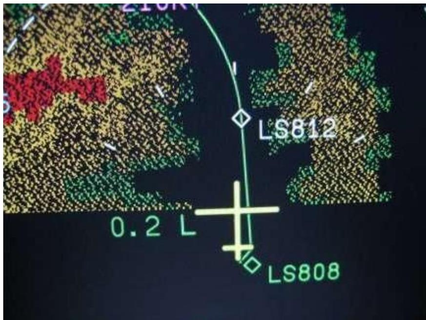
Fig 7.2: Example of cross-track deviation display in 1/10<sup>th</sup> NM
