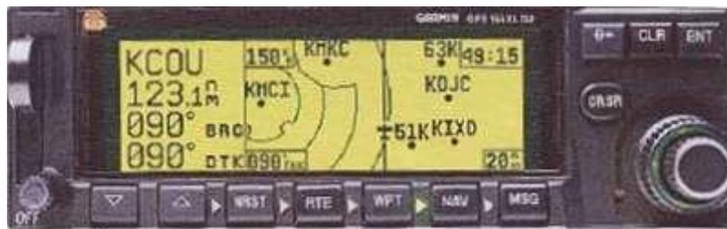
Figure 2.4: Typical Stand-alone GNSS Receiver
