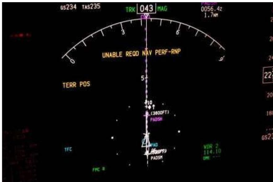
Fig 4.1: Alert annunciated on Boeing 737NG navigation display
